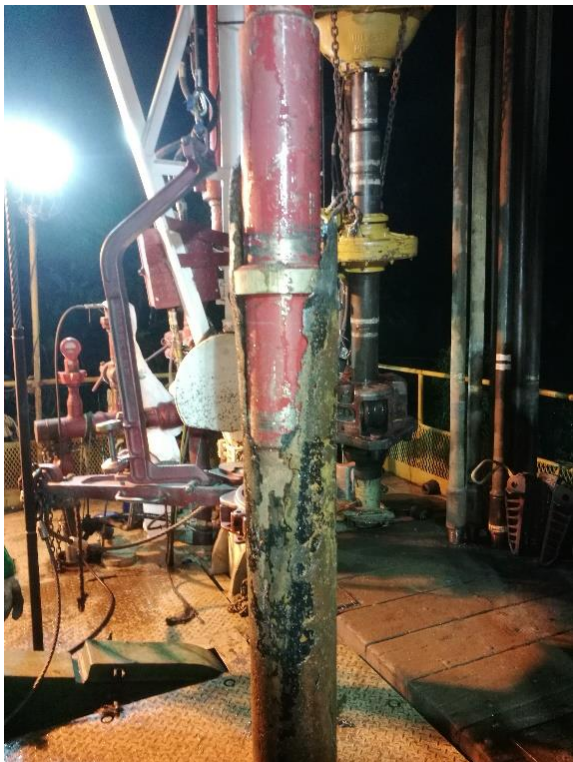
Figure 8: A section of Bul-25's hangdown liner showing extensive corrosion.
