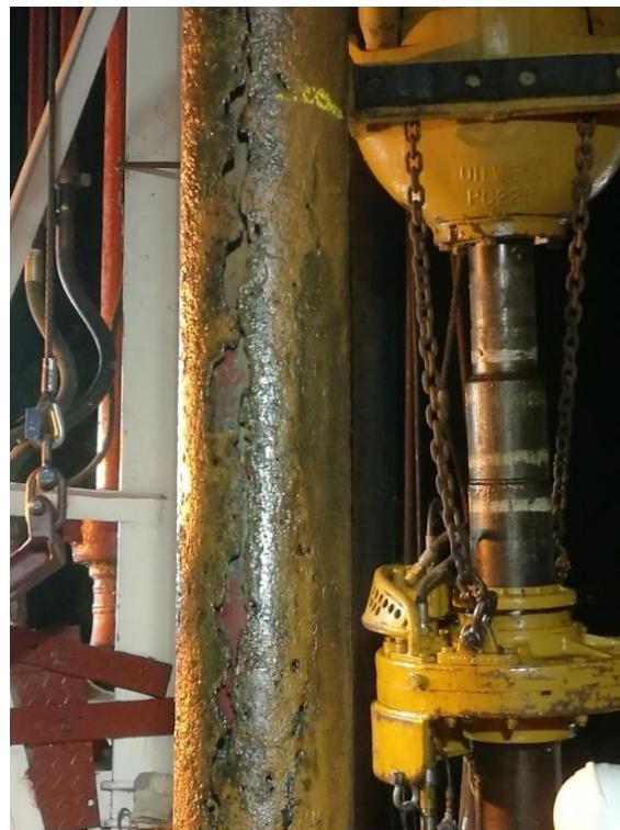
Figure 9: A section of liner approximately located at 800 ft MD (243.8 m MD) showing streaks of corrosion and pittings.
