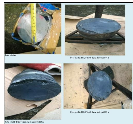
Figure 4. Impression block tool profile
