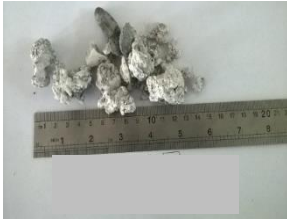
Figure 6. Scale in production well
