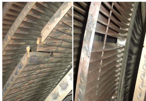
Figure 6: Blading failure and subsequent repair to get back in service till rotor can be rebladed. Blade on opposite side was cropped to keep it in balance.
