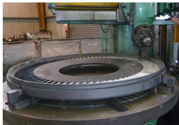
Figure 8: Machining a diaphragm after repairs and metalspray to ensure correct clearances are maintained.
