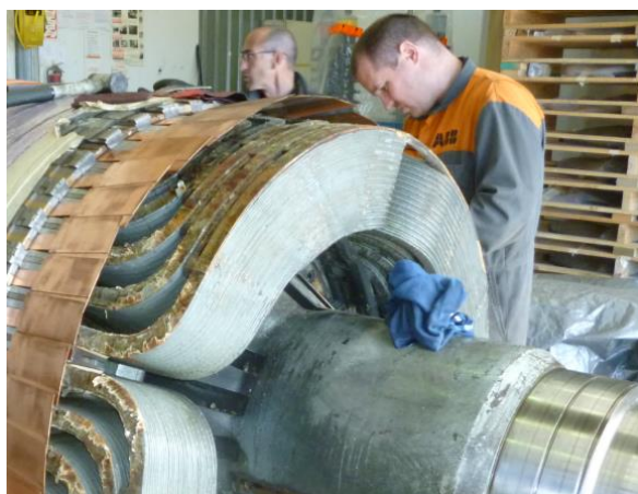
Figure 7: 30MW generator rotor being worked on during endring inspection. Segmented amortisseur and original mica insulation visible.
