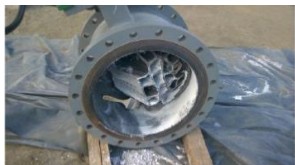
Figure 13: Steam valve with silica scales
