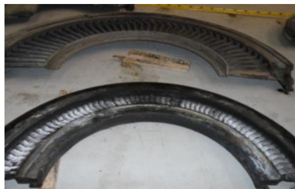
Figure 12: Turbine blades with silica deposits on nozzles from Olkaria II
