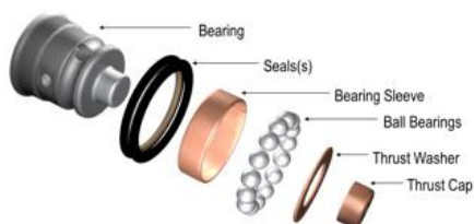
Figure 11: Bearings inside a roller cone bit
