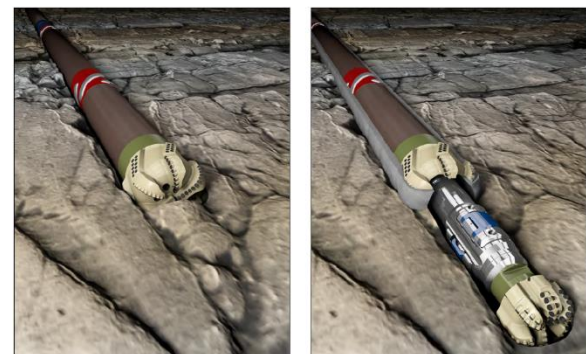
Figure 23: The casing bit can be drilled out after the casing has been cemented at the TD
