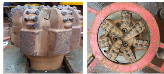
Figure 22: 9.875-in CDE bit post run condition
