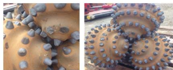
Figure 28: 24-in bit dull grading (2-3-BT-A-E-1-WT-TD) after pulled out of hole with based BHA
