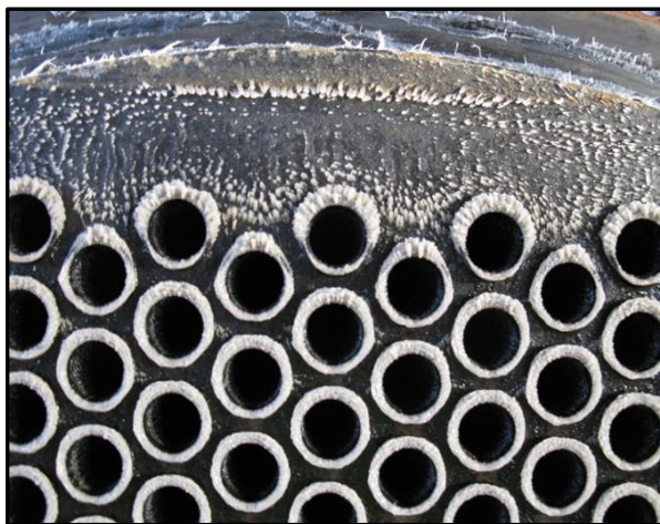
Figure 3: G16 pre-heater end cap tubes coated with silica scales as inspected in May 2016.
