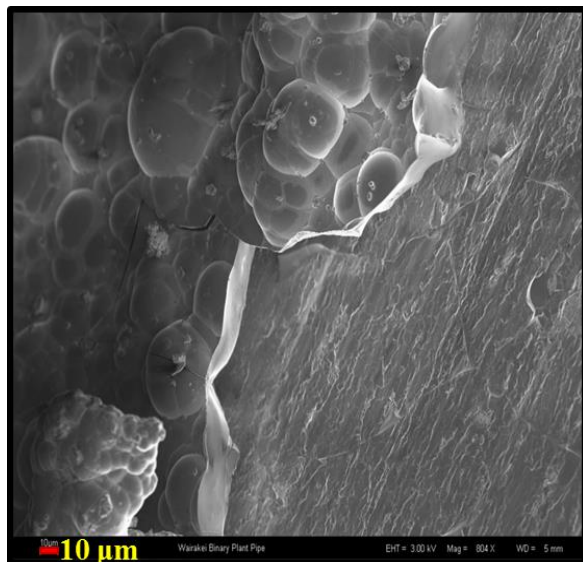
Figure 6: SEI analysis showing coalesced spherules of amorphous silica (40-50 µm dia.) after Zarrouk et al. (2014). Samples collected at the Wairakei Binary Plant before GEO981 dosing was conducted.
