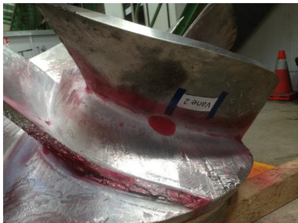
Figure 7: Unit 2B HWP impeller failure.
