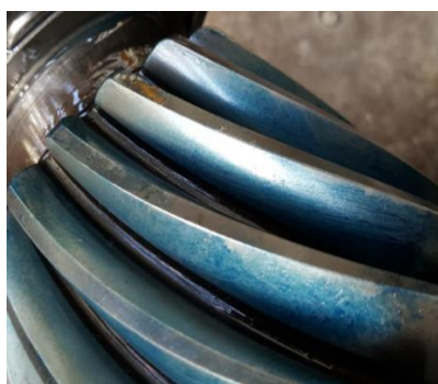
Figure 5: Original pinion drive face (concave) showing different contact pattern from flank to flank.
