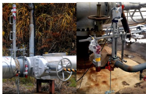
Figure 13 Setting up of Gamma-ray pipe section profiler (GPSP) in the field
