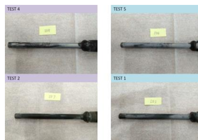
Figure 17 Okuaizu1: The surface of Corrosometer® Probes (CS) after testing
