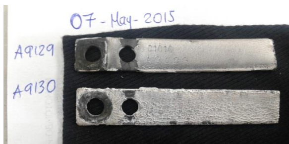
Figure 8: Scale coupons at inlet and outlet of OEC after 5 months.
