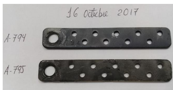
Figure 11: Scale coupons 10 months into the new program
