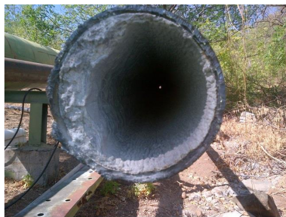
Figure 4: Scale in pipeline of Separator Brine Line
