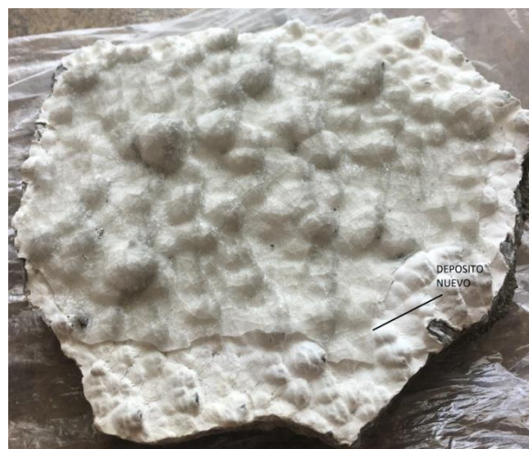
Figure 12: Old scale deposit with newer deposit having coated on top. Old deposit is dark grey material almost 1/2 inch thick. New white deposit was only 1/64" thick.
