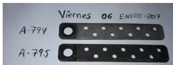
Figure 10: Scale coupons three weeks into the new program
