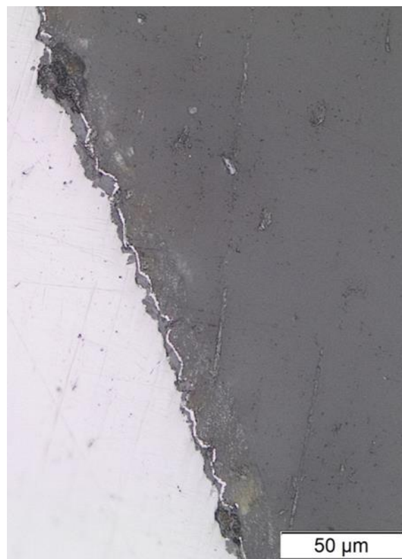
Figure 7: Metallurgical cross section (prepared at a 45° angle) of heavy metal deposited layer on carbon steel sample exposed at pH 3.8 after 4 days in Test2.
