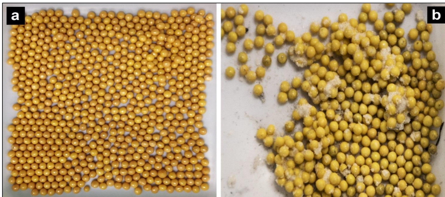
Figure 3. Photographs of a) unreacted zirconia ( \text{ZrO}_2 ) beads, ~2 mm dia; b) zirconia beads collected at the bottom of the preheater after the experiment. Note the extensive precipitation of secondary mineral material.
