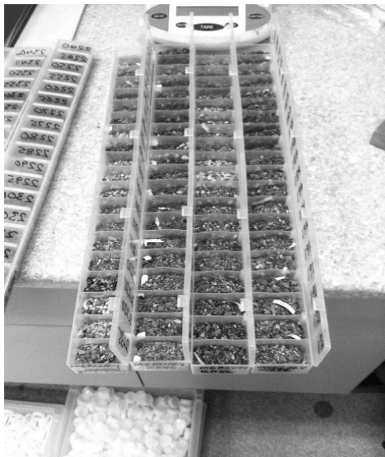
Figure 2: Drill cuttings from the Kawerau greywacke basement; change in color reflects argillite/meta-sandstone compositions.
