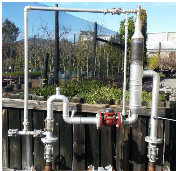
Figure 4: Flow loop + separator + inline meter; rig design for roll-out of trial implementation.
