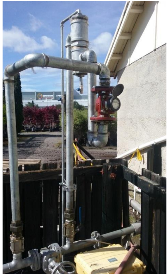
Figure 9: Trail construct - flow loop with separator prior to inline flow meter.
