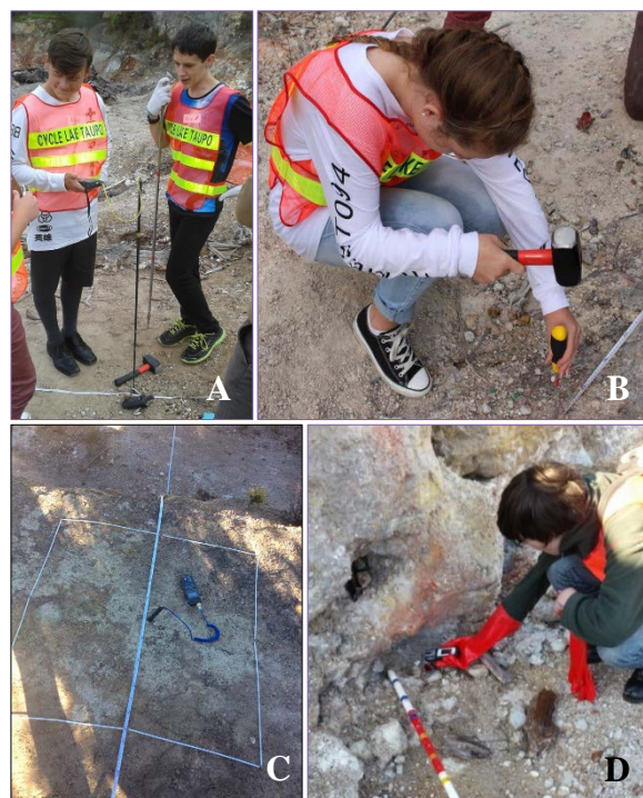
Figure 4: Taupo College students undertaking various geothermal monitoring activities at Crown Park thermal area. A. Measuring 1 m depth soil temperature profiles on a transect line; B. Using a screwdriver and mallet to create a hole for measuring 20 cm depth soil temperature on a transect line; C. Use of 1 m square quadrat to record ground cover. D. Measuring gas concentration at an active fumarole.
