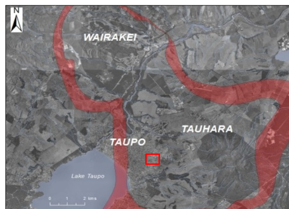
Figure 1: Location of Crown Park thermal area (denoted by red square) relative to the Wairakei-Tauhara geothermal field (outlined by the resistivity boundary (red shading) as defined by Risk et al., 1984).
