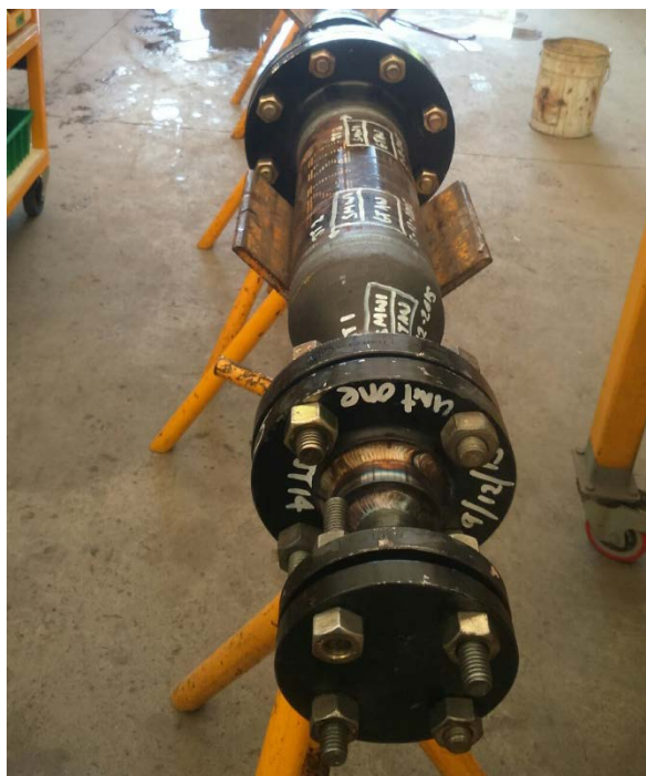
Figure 3: Fabrication of coupon unit
