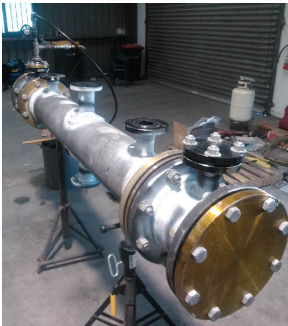
Figure 1: Setting up the shell and tube heat exchanger rig for hydro-testing
