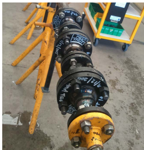
Figure 2: Fabrication of the double pipe heat exchanger units
