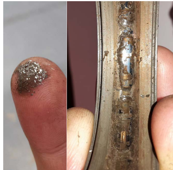
Figure 8 - Left: Example of metal flakes found in bearing housing. Right: A section of the outer race of the seized bearing.
