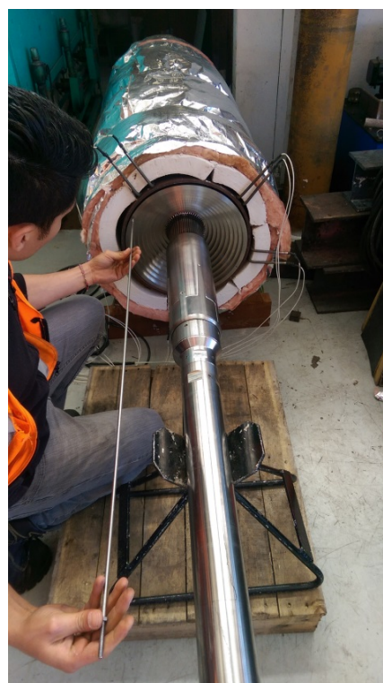
Figure 4: HTCC-MF being loaded into calibration oven.
