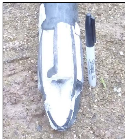
Figure 12: Anhydrite scales on the monitoring well pressure chamber (set depth: 1650 m measured depth)
