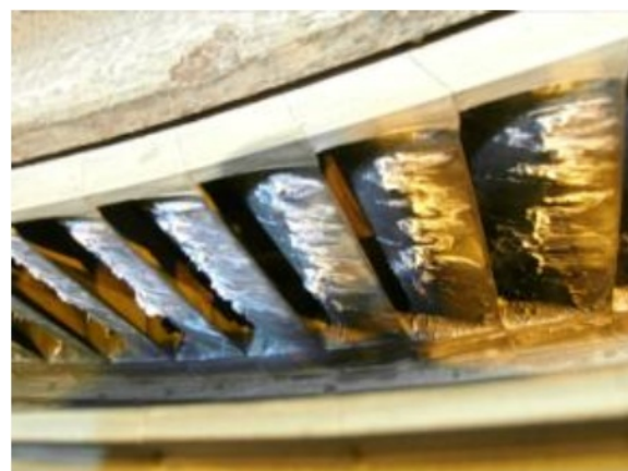
Figure 1: Mineral Deposition on a Turbine Diaphragm at Wairakei Power Plant (from Morris and Robinson, 2015).
