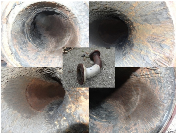
Figure 11: Well 1 branch-line sweep bend inspected on June 2013, showing significant erosion damage.
