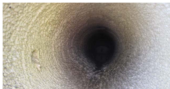
Figure 21: Common silica scaling on a pipe wall.
