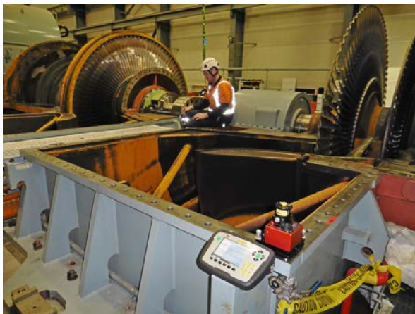
Figure 9: Measuring Casing Flatness
