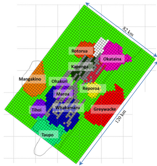
Figure 3 The areal grid structure of the model and initial rock type distributions at -700 masl (Layer 3) with faults representing the TFB (grey)
