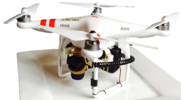
Figure 1: DJI Phantom quadcopter modified with ICI thermal camera
