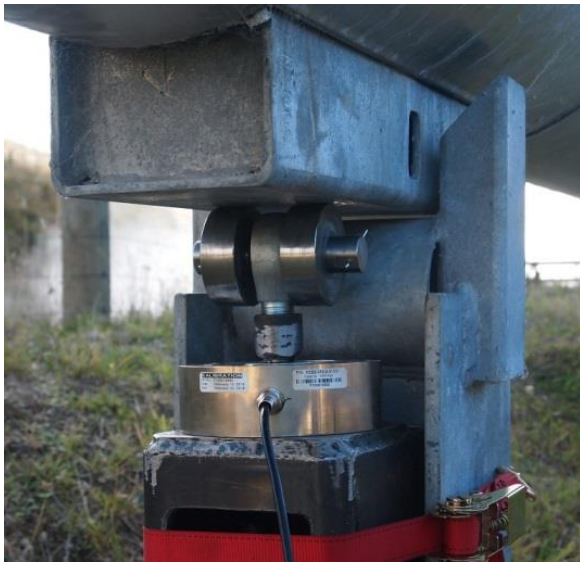
Figure 4: Load cell detail. Note small air gap between shoe and pipe support, showing that weight of pipe is on load cell and not pipe support.
