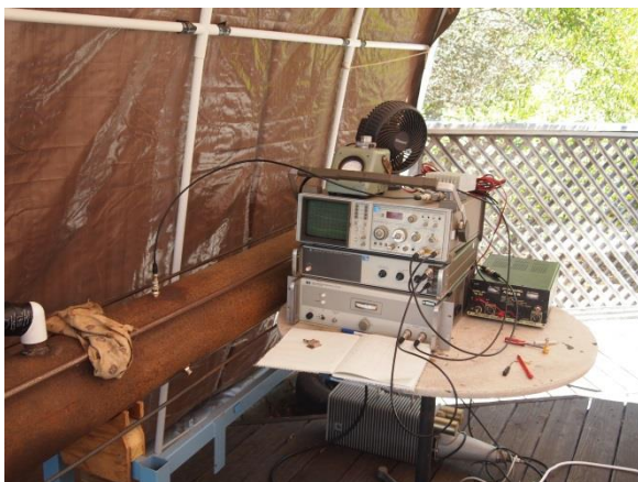
Figure 3: Test setup, using an 8 inch internal diameter steel pipe.
