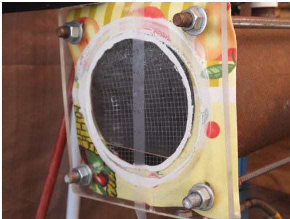
Figure 7: Linear scale, shown on vertical tape added to face of view port.
