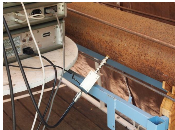
Figure 5: Receive antenna and preamp, mounted into pipe at 45 degree angle.
