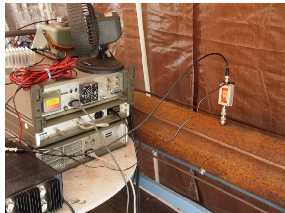
Figure 4: Receive antenna and preamp mounted vertically into pipe from top.
