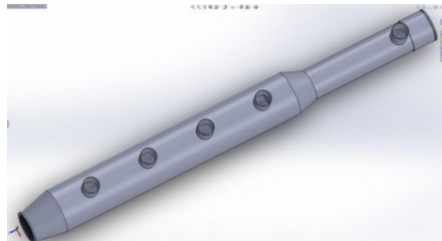
Figure 7 - CAD model of the pentane vaporizer
