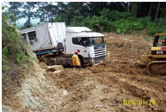
Figure 2.3: Muddy terrain is a common issue encountered in rig mobilisation during the rainy season.
