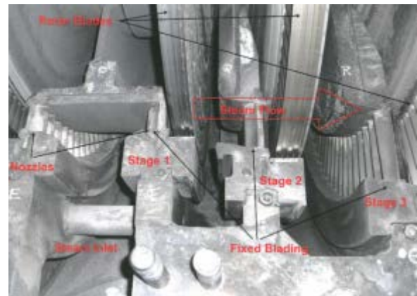
Fig 2 Turbine nomenclature used in this paper. A stage is a set of fixed and rotor blades. The nozzles are the first stage's fixed blading. The vanes are the individual blades in the fixed blading.
