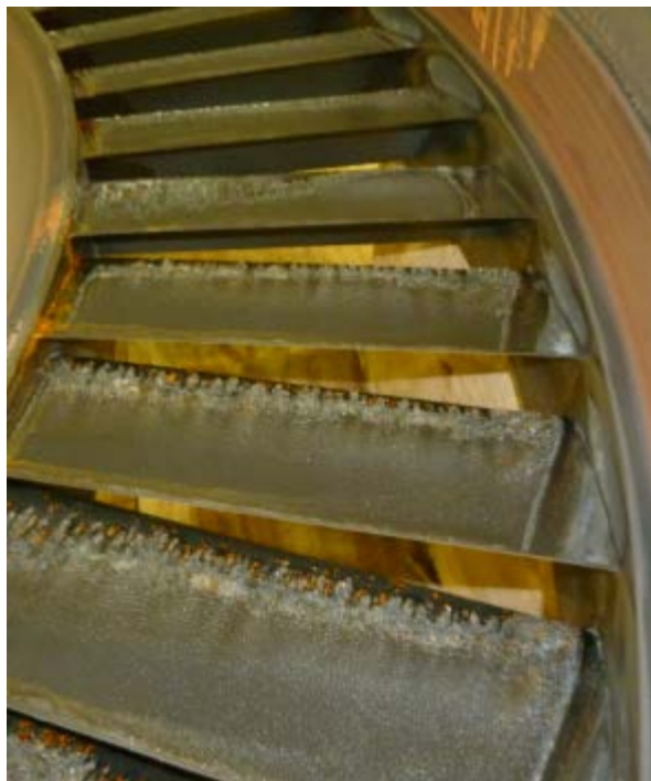
Fig 8: Effect of wet steam - minor deposition on the vanes, mainly silica, and clear areas from water flow at the port walls. There has been post shutdown redissolving of solids so corrosion has started.
