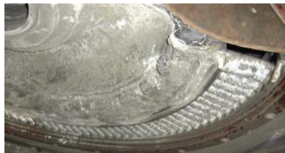
Fig 7: Deposition in the turbine nozzles and casing. This is because the mineralised fluid coming through the nozzle is about saturation. The water flows into the cavity upstream of the first stage rotor blades. Here it is heated by heat flow through the steel from the higher pressure steam. The water evaporates, leaving the minerals behind.
