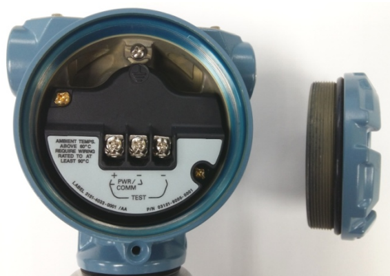
Figure 1: Hermetically sealed termination area, isolating the termination from the electronics. Also note the o-ringed sealed cap.
