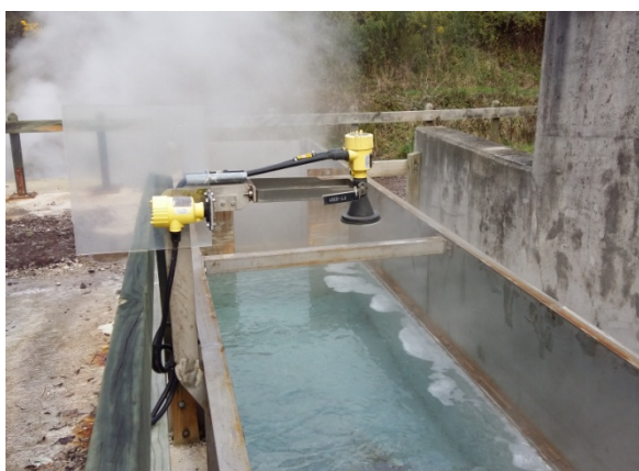
Figure 3: Non-contact radar measuring weir flows. Note the remote display and removable bracket.
