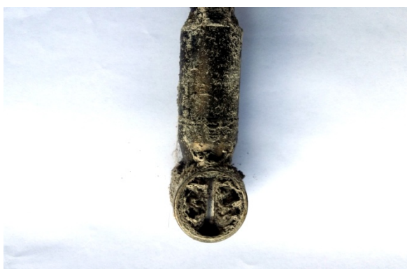
Figure 2: Vortex shedder bar blocked with scale due to use in geothermal brine.
