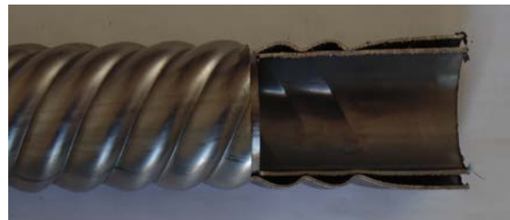
Figure 1 Photograph shown spiral flute co-axial tube construction technique
