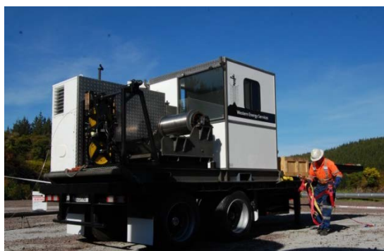
Figure 2: Slickline skid unit containing .108" slickline, counter, tension device, hydraulic motor, and control cabin.
