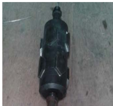
Figure 3: Diamond style broach used for harder calcite or silica.
