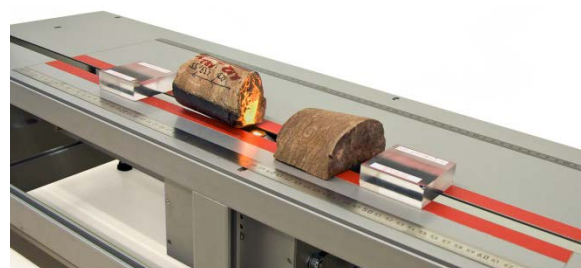
Figure 2: Thermal Conductivity Scanner with two rock samples and two standards made of fused glass.
