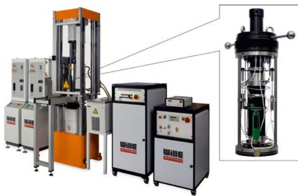
Figure 3: The Thermo-Triax test rig.
