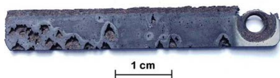
Figure 5 Carbon steel (A106-B Grade) mass loss coupon (flat strip) exposed to well X6D fluid for 14 days. The coupon was inserted inside the two phase pipeline of the well using a retractable coupon holder. Note the large corrosion pits on the surface of the coupon. The coupon edge facing the downstream flow of the fluid is eroded.
