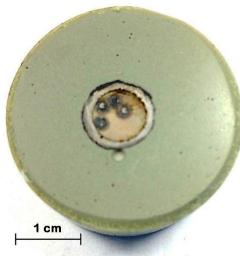
Figure 6 Cylindrical ER probe cut across the diameter and mounted on resin and polished. Note the wire and ceramic inside the probe. Scale and corrosion products line the outer wall of the probe.
