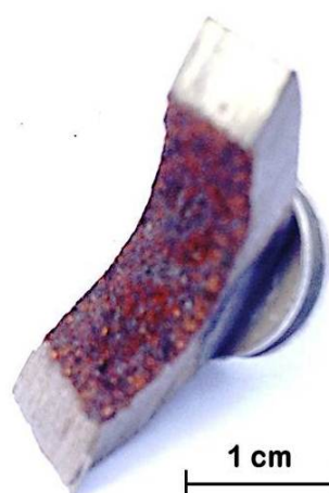
Figure 7 A small section (about 1 cm long) was cut from the pipe in Figure 2 and attached to a stub mount. The inside surface of the pipe is covered with about 1 mm thick corrosion product.
