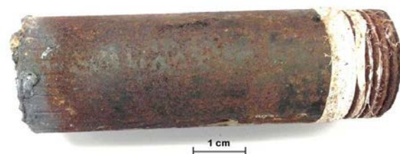
Figure 2 Carbon steel pipe (1") used to transmit X2D fluid for 1 month at low flow condition. A section of pipe was cut near the thread (Figure 7). The inner surface of the pipe is coated with corrosion product and scale.
