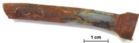
Figure 3 The sample above is the remaining piece of a cylindrical ER probe used to monitor well X6D corrosion rate. After 10 days of exposure half of the probe was cut due to corrosion.
