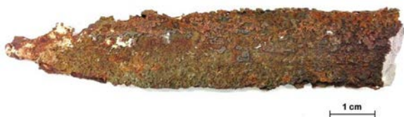
Figure 4 A piece of 4" diameter carbon steel pipe used as a capillary tubing stinger inserted into well X6D. More than half of the stinger has been lost due to corrosion before it was retrieved.
