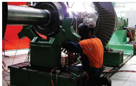
Figure 3: Turbine refurbishment underway at AIE workshop, Kawerau, NZ (NZTE Geothermal companies' profiles, 2014)
