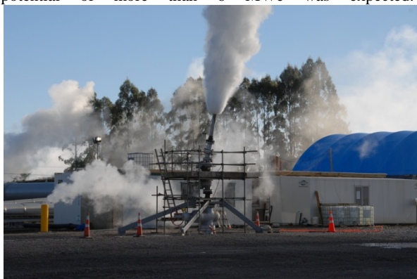
Figure 6: Vertical discharge being conducted in the middle of the construction site.
