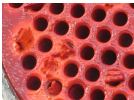
Figure 8. Soft paste-like deposit after dosing 20 ppm
