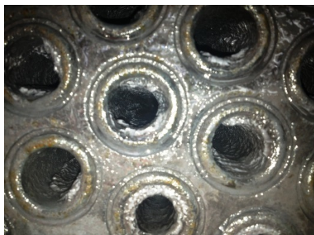
Figure 7. Soft paste-like deposit after dosing 4 ppm
