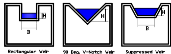
Figure 15: Typical weir box with several types of discharge shape side.
