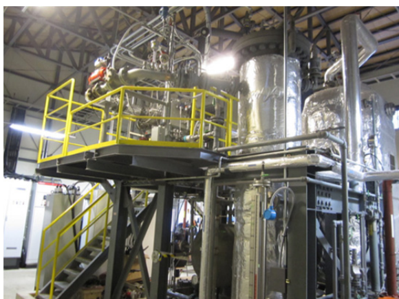
Figure 6: The Kalina power generation system using hot spring fluid at Matsunoyama.
