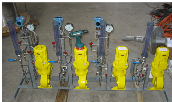
Figure 2: Four-pump dosing skid prior to installation with a stinger in the background
