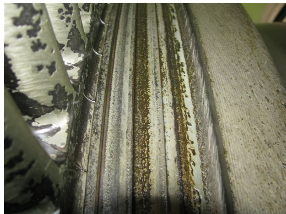
Figure 9. Corrosion of a turbine rotor seal – note the silica deposition on the rotor blades.
