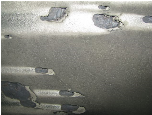
Figure 3. Corrosion damage on a geothermal steam pipe downstream of a wash water injection station. At this plant the wash water is oxygenated, while the steam contains hydrogen sulphide.
