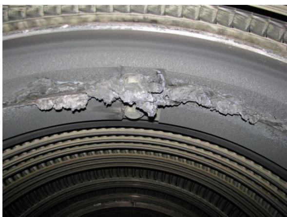
Figure 6. Solid particle erosion on HP and IP turbine nozzles as a result of heavy silica deposition and resultant transport through the turbine.
