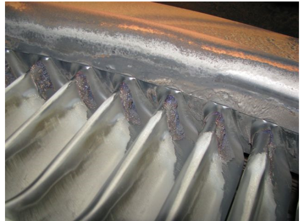
Figure 5. Iron sulphide deposition on steam turbine nozzles – the iron sulphides result from the corrosion of the steam path due to the presence of H_2S and moisture.
