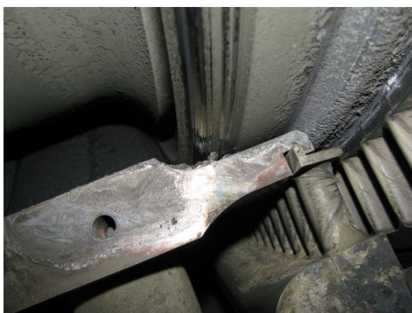
Figure 8. Metal loss suffered from a steam turbine due to hard silica deposits becoming wedged between the turbine rotor and casing.
