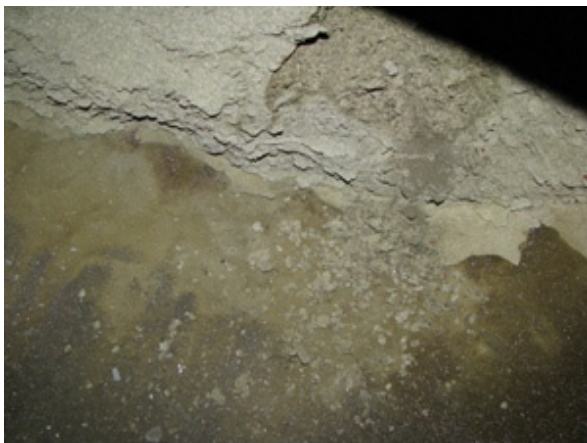
Figure 4. Corrosion product deposition within a high pressure steam strainer.
