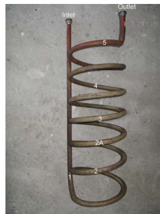
Figure 3:- The locations at which the coils were cut for subsequent analysis.
