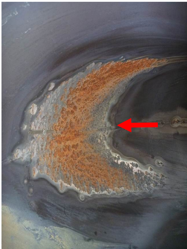
Figure 4: Example of localized metal loss inside elbow. Approximate dimensions are 20x30cm. Flow is indicated with the red arrow (Amend and Yee, 2012)
