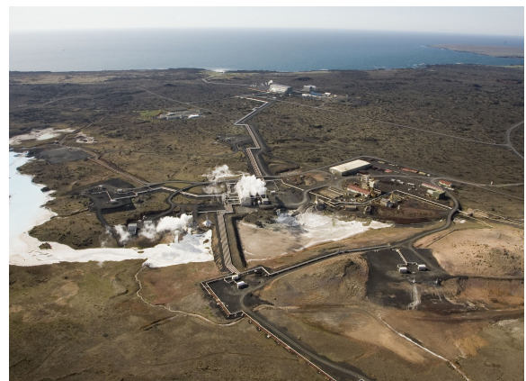
Figure 4: The photo shows the Reykjanes well field and the 100 MW e power plant in the background. A tentative site for well IDDP-2 is in the area to the right of the steam separation house in the middle of the photo. That siting, as well as the drillhole design, is now being re-evaluated.
