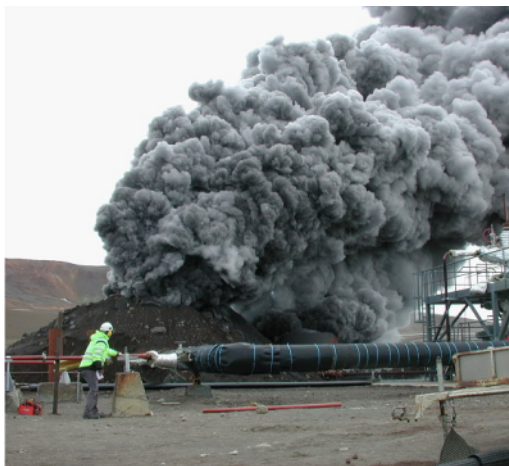
Figure 2: Dark colour at the beginning of each flow test, due to casing corrosion, lasts for about 5 minutes, then the steam turns transparent and superheated as in figure 3.
