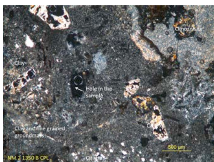
Figure 5: Photomicrographs using cross-polarized light of NM2.
