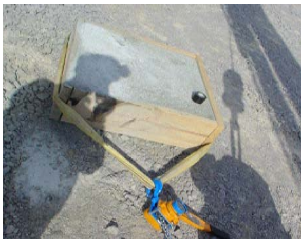
Figure 2.5.1: Concrete Test Block on Crushed Rock
