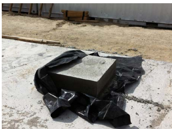
Figure 2.5.2: Test Block on Polyethylene
