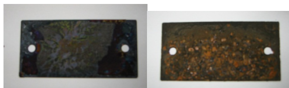
Figure 4: Photographs of corrosion on the Cu plate and the iron plate.
