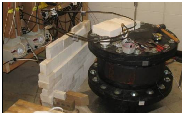
Figure 1: Heated true-triaxial cell with sample installed.
