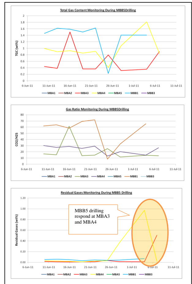
Figure 6: Graph of gas monitoring trend versus time during MBB-5 drilling.
