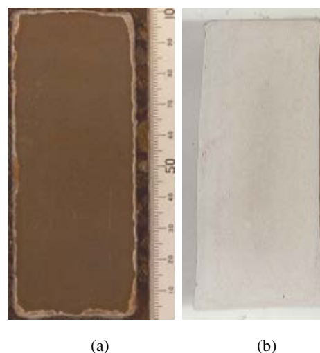
Figure 2: Exposure of grout cylinders in BR17, Ohaaki (260°C, [CO 2 ] 0.064 moles/l, pH T 6.49) for 6 months
