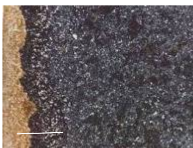
Figure 4: Photomicrograph of carbonated geothermal cement sample from Fig 3.
