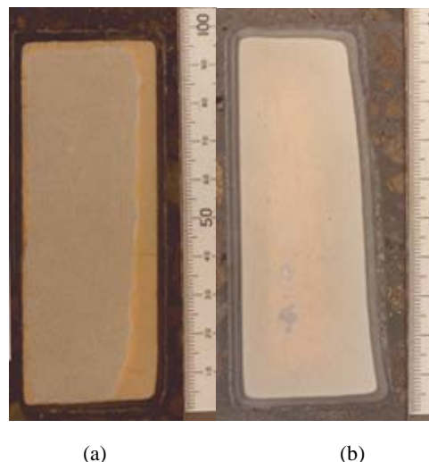
Figure 1: Exposure of grout cylinders in BR23 Ohaaki (150°C, [CO 2 ] 0.35moles/l, pH T 4.59) for 6 months
