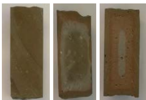
Figure 6: Grout formulations containing 25% Microsilica WG at different densities cured at 150°C
