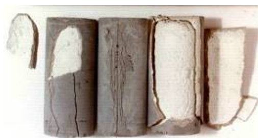
Figure 3: Exposure of pure cement samples in BR17 at 260^\circ\text{C} for 4 months
